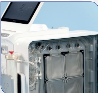
Dialysate cassette automatically supported
